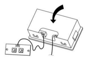
Connect the power cable (24V DC Power Supply). The 3V battery is replaceable.
